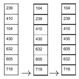
We start off with an unsorted list then we move every item into buckets based off their highest digit. The way we order within buckets is based off relative position in the list from the previous iteration. After 2 iterations, every item is in its own bucket so the algorithm terminates.
